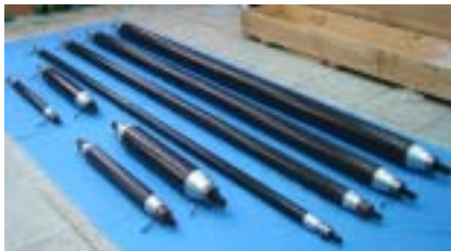
(a) CFRP tubes for latticed space structures
