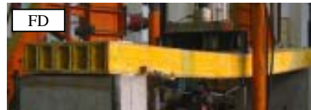
(a) FRP deck without outside filament winding
