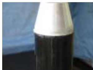
(c) Debonding failure under compression
