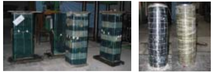
(a) Specimens of confined RC columns: square and rectangular section confined with CFRP and hybrid FRP; GFRP and hybrid C-G-FRP tube
