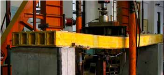
Figure 2 Test of an all FRP deck
