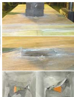
Figure 6 Punching of HDW3 Figure 7 Load-deflection curves in Case 2
