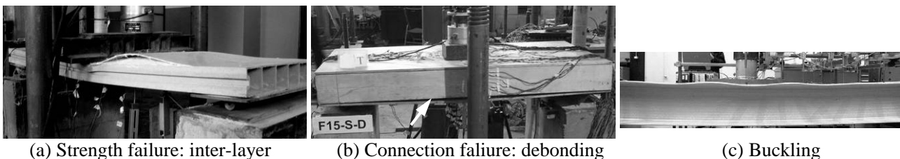
Figure 1 Failure modes of FRP decks
