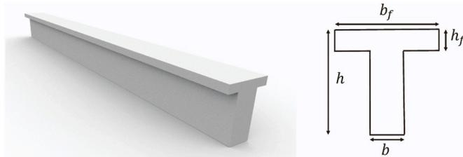
Where  $L$  is clear span length;  $S$  is beam spacing;  $h$  is overall beam depth;  $b$  is web width;  $b_f$  is top flange width;  $h_f$  is top flange thickness; DL and LL are dead load and live load;  $A_s$  is cross-sectional area of longitudinal reinforcement;  $A_{sv}$  is cross-sectional area of shear stirrup;  $M_u$  is flexural capacity;  $V_u$  is shear capacity; and  $RF_M$  and  $RF_V$  are flexural and shear performance rating factors, respectively.
