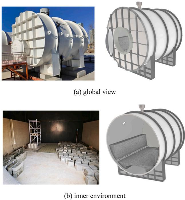
**Fig. 1.** Sealed tube for vacuum exposure.
