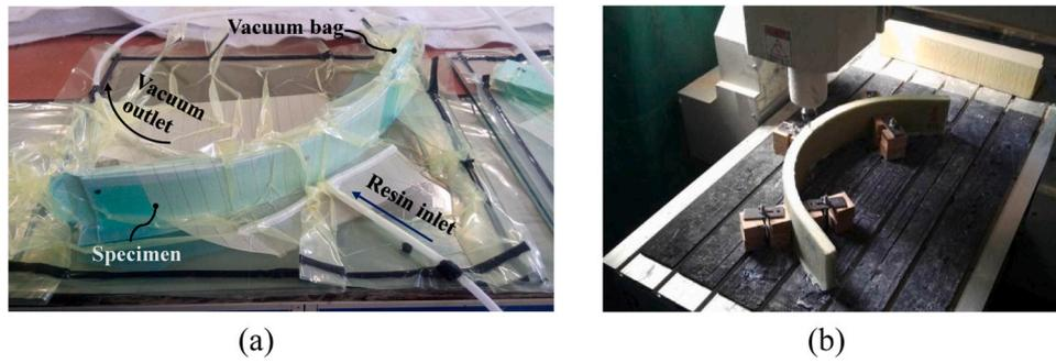
Fig. 2. Manufacture process of singly curved GFRP sandwich panel with foam core: (a) VARTM process and (b) CNC machining.
