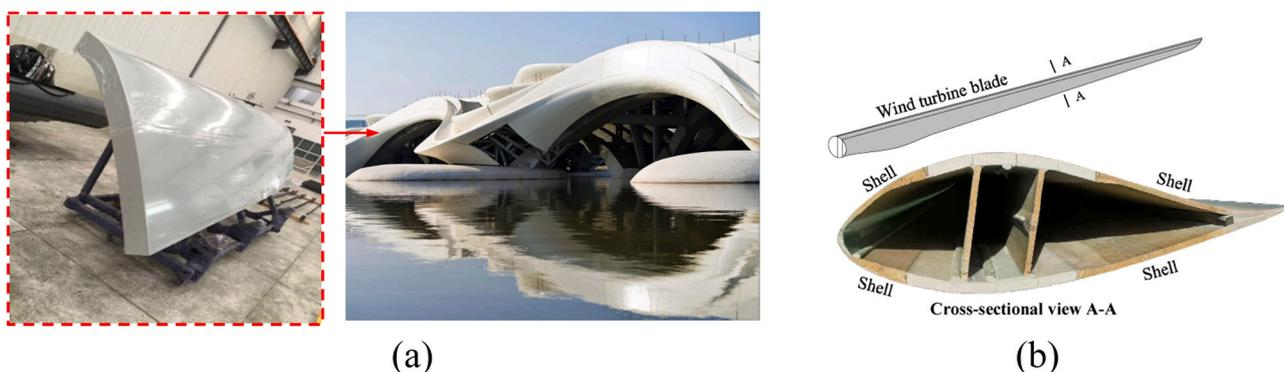
Fig. 1. Curved GFRP sandwich panels as (a) the envelope of a bridge (Beijing, China) and (b) the shell of the wind blade.
