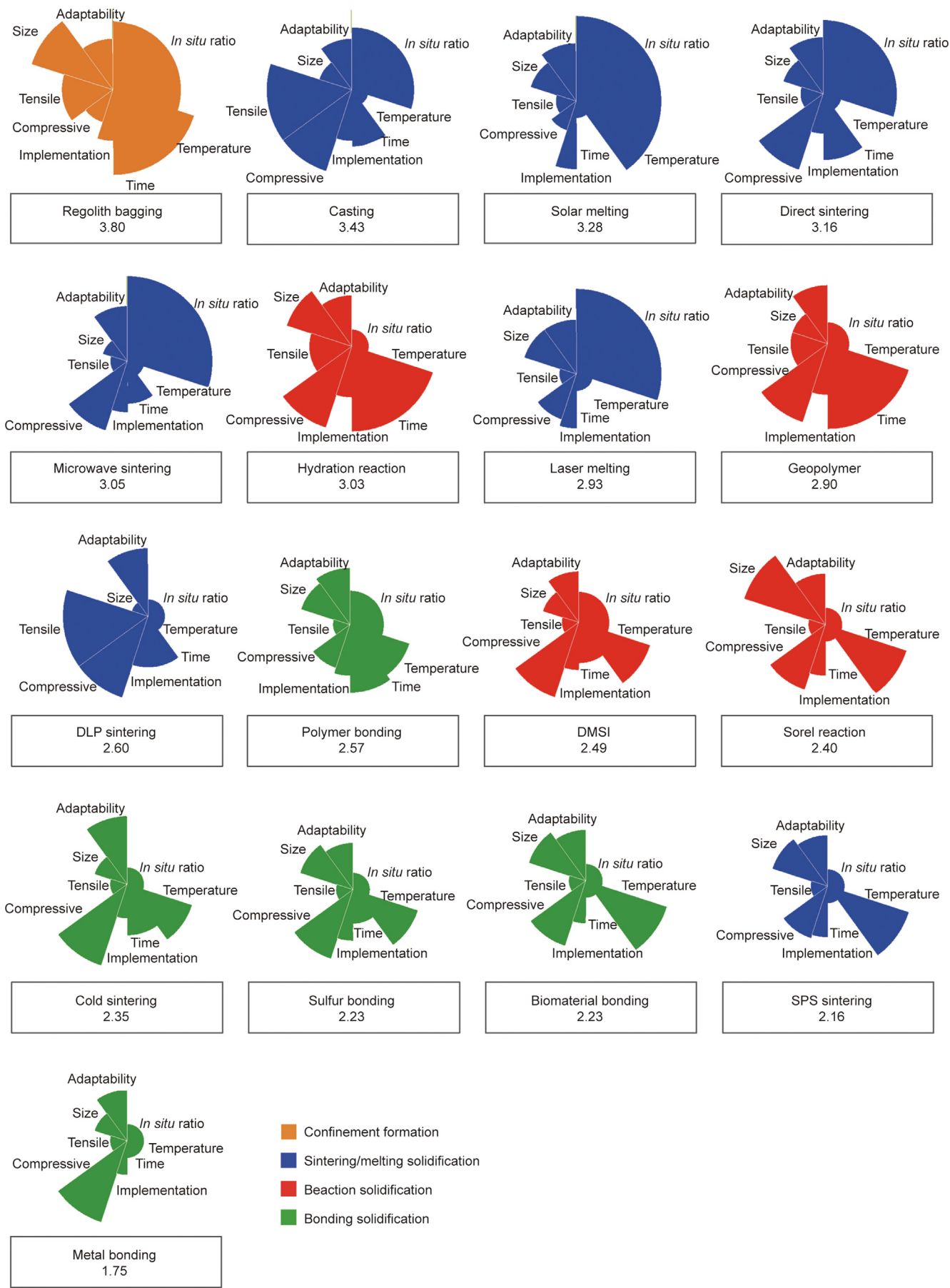
Fig. 9. Scores for lunar regolith solidification and formation strategies. The techniques are sorted by score. Regolith bagging is the highest-rated technical solution, followed by casting, solar melting, direct sintering, and microwave sintering.
