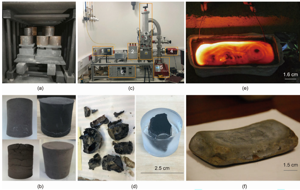
Fig. 3. Sintering solidified instruments and specimens: (a, b) direct sintering [34]; (c, d) microwave sintering [35]; and (e, f) self-propagating sintering [36]. Reproduced from Refs. [34–36] with permission.
